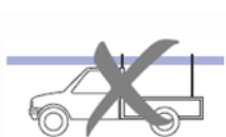
Load too large for vehicle, projecting too far from front and rear
