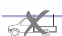
Load too large for vehicle, projecting too far from front and rear
